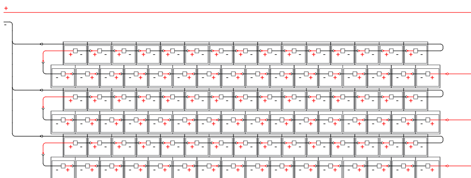
Wiring diagram for the system with SOLAR FLAT-5XL ceramic roof tiles
