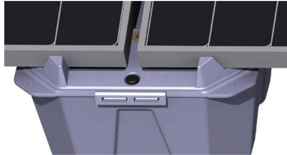
**Recommendation:** Put the first and last LANDBLOCK® on every row in the area and run a line from the first lug to the last one to use as a guide for levelling and lining up the rest of the LANDBLOCK®.
