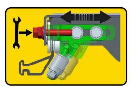
Anti tip mechanism for sliding tray.
