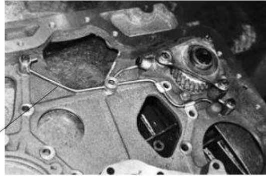
Fig 5-24 Lubricating Pipes Installation
